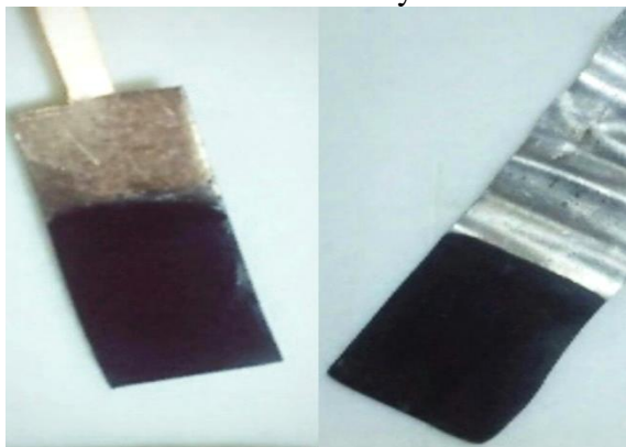
Figure 16. Examples of thin layers obtained on copper (a) and platinum (b) electrodes in the Re – Se – Cu system.
